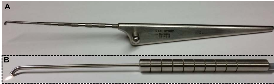
Figure 6.2: Similarities between conventional arthroscopic hook used by surgeons (A) and custom designed NIRS optical probe (B) used in study III of this thesis.
